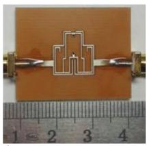
▲ Fig. 7 Photograph of the fabricated tri-band filter.
